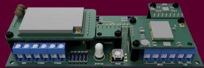
Designed a **custom PCB** and a **communication protocol software** for the avionics bay
